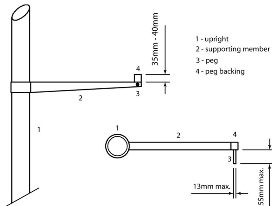
**Figure (b) TR28 (Rule 183) - Pole Vault crossbar support**
