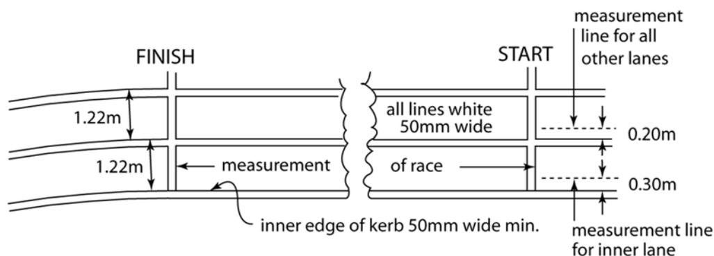
**Figure TR14 (Rule 160) - Track measurements (infield view)**
